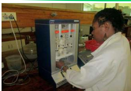
Quality Control Chemist, carrying out food testing on the Fat extraction equipment
