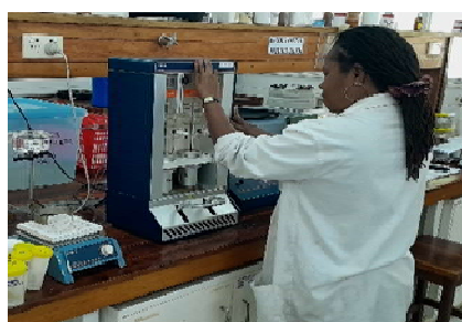
Extraction technique to extract from crushed, dried or ground samples with the aid of heating & refluxing to determine fats in dried nuts, grains, etc
