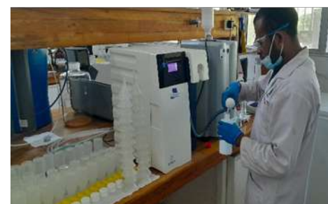
This is a purification system which eliminates bacteria using ultra violet radiation and provides chemical reactive water for the laboratory's daily use.
