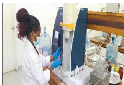
Unit used to determine nitrogen (crude protein) content in soil, plants, food and natural products.
