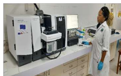
A high throughput & inexpensive analytical technique used to primarily test for major elements such as Calcium, Magnesium etc in food, beverage, water, plant and soils.
