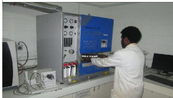
Carbon Sulphur test using CS Analyzer
