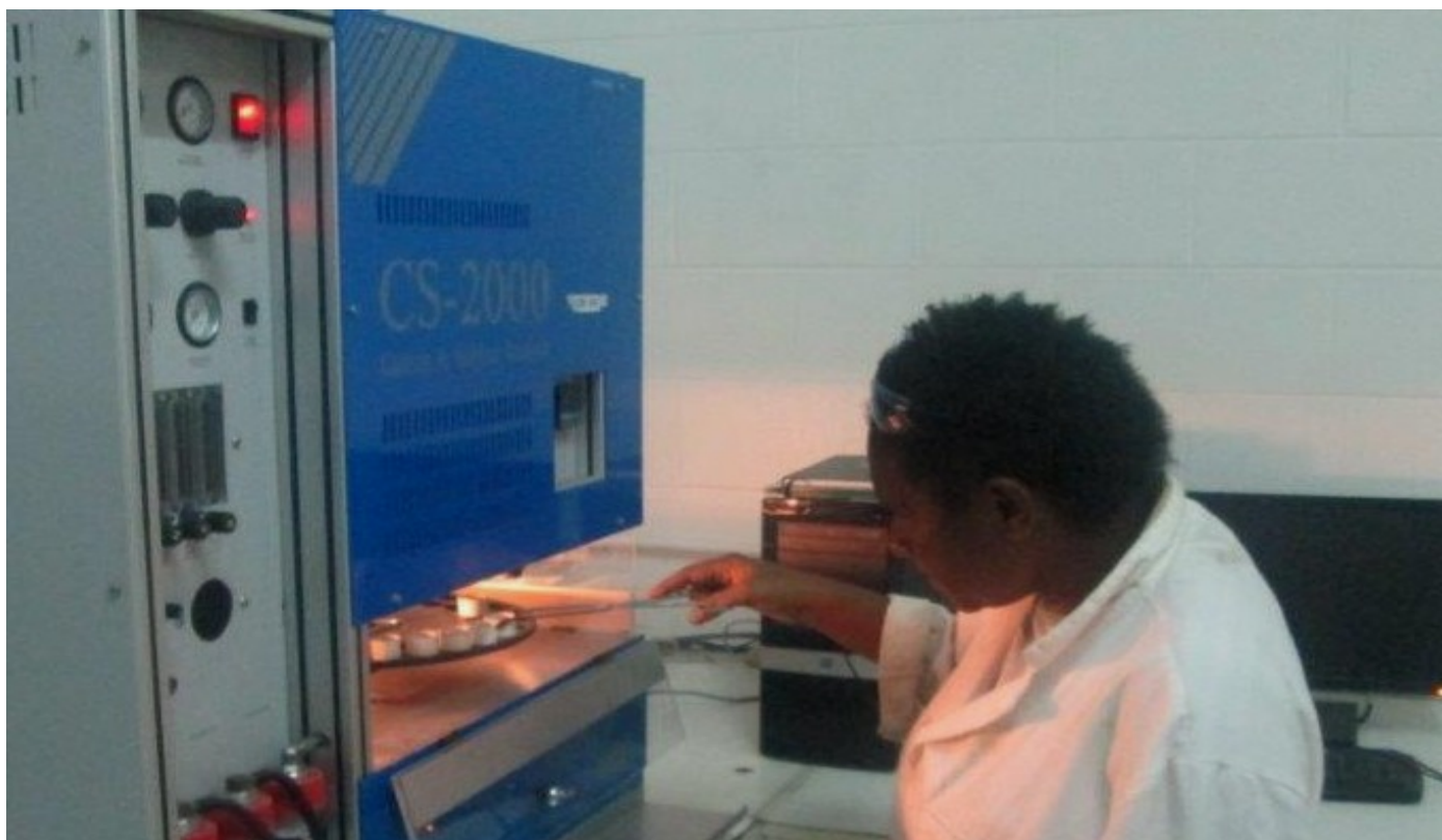
Carrying out soil test using Carbon Sulphur Analyzer.
