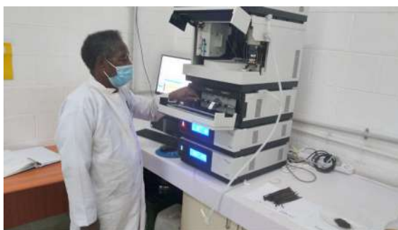
Preparing the new Ultra Liquid Performance Chromatography ready for Vanillin test on Vanilla beans
