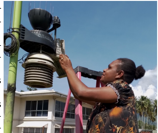
Replacing battery of the automated weather station.
