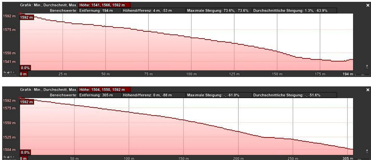
Fig: 11: Elevation profile of existing pipe 2 (above) and proposed extension of pipe 2 (below)
