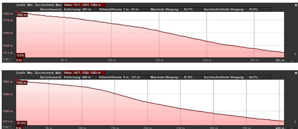
Fig: 10: Elevation profile of existing pipe 1 (above) and proposed extension of pipe 1 (below)
