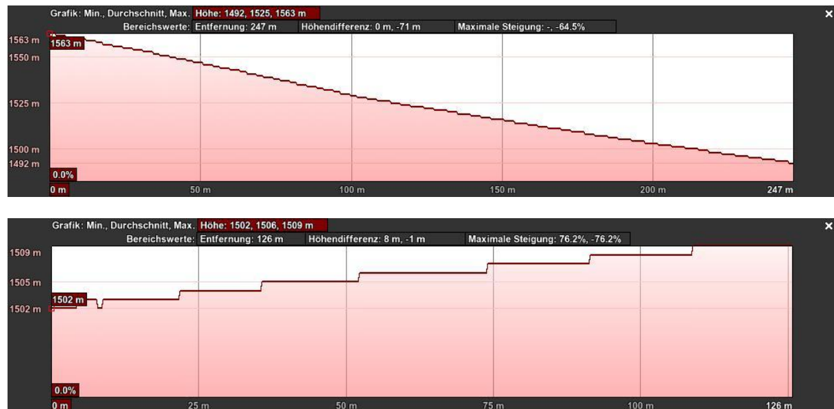
Fig: 13: Elevation profile of proposed down pipe (above) and delivery/supply pipe (below) for ram pump
